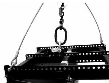
Fig. 29: Secondary safety - Type 2
